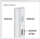
Position the new bottom strike closer to the interior. You may need to chisel out your strike hole and pocket so that the new strike will sit flush.
